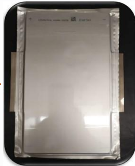
Single EnerDel Waste Lithium-Ion Battery from EV
