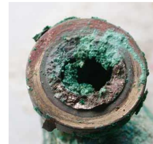
Corroded water pipe
